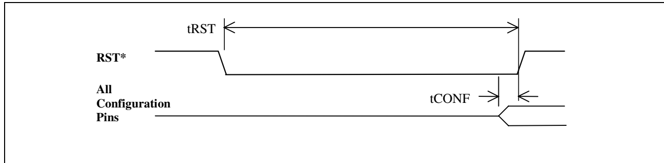
Figure 6: Power on Reset
